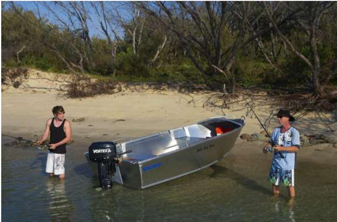
The 385 Big Boy now features 2mm top and bottom plate sides, which adds an extra element of toughness to the already solid design.
